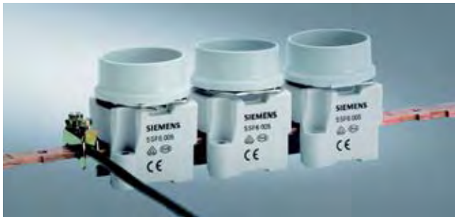
DIAZED 5SF6 005 bus-mounting base DII for 25 A with terminal version "B" mounted onto an EZR 5SH3 54 busbar. The feeding conductors are clamped to the 8JH4 122 bus-mounting terminal. The busbar has a load capacity of up to 150 A.
