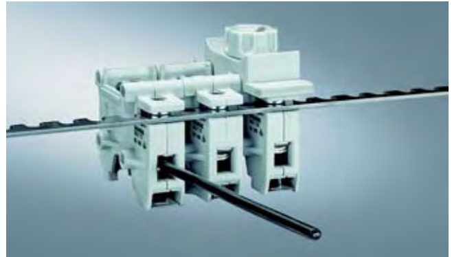
NEOZED base D01 for 16 A, 5SG1 330 with terminal version "R", mounted onto a 5SH5 321 busbar in fork-type version, non-insulated. The busbar has a load capacity of up to 116 A.
