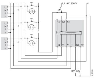
The device is fitted with a direct voltage input for the control of an 5LZ....-4 ECG dynamic. When the pushbutton is actuated, the power supply is released and the ECG dynamic is brightened, depending on the setting of the time switch, for up to 10 minutes.
