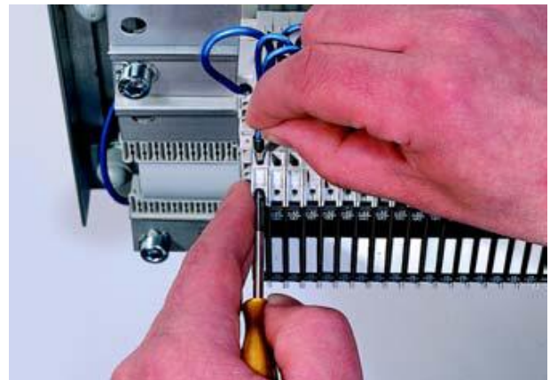
Connecting a lead to the spring-loaded terminals
