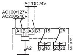
Pulse-forming with auxiliary voltage
