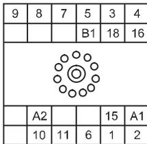
**7PX9 921 socket for 7PV33 timing relays**
