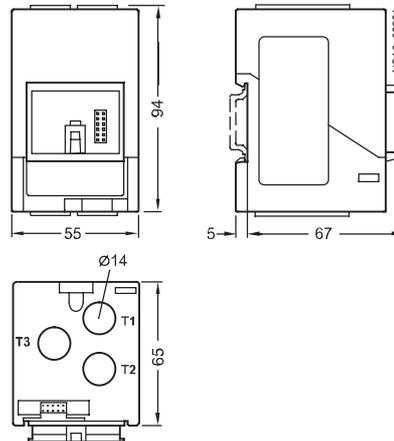
3UF7 103 current measuring module (straight-through transformer)
