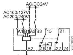
Pulse-forming with auxiliary voltage
