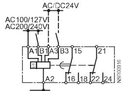
Additive ON-delay with auxiliary
