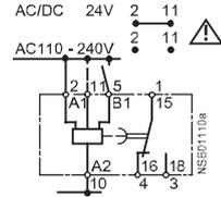
OFF-delay with auxiliary voltage (C)
