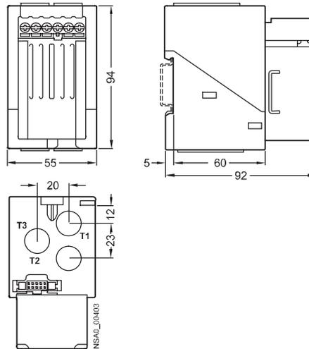
**3UF7 113 current/voltage measuring module (straight-through transformer)**
