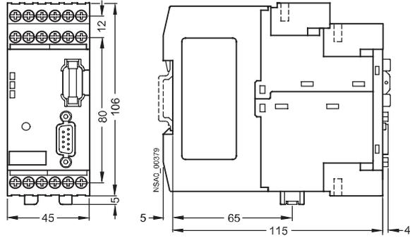
3UF7 100, 3UF7 101 current measuring module (straight-through transformer)
