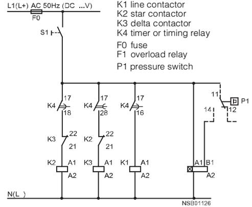
The contact element 17/18 is only closed in the star stage; the contact element is open in the delta stage as well as in the de-energized state.
