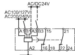
OFF-delay with auxiliary voltage
