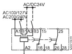
OFF-delay with auxiliary voltage
