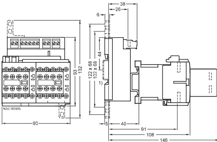
3TK28 52, 3TK28 56 with spring-loaded terminals
