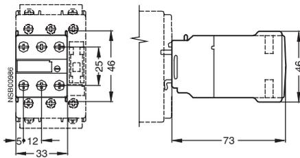
**3RT19 16-2C solid-state time-delay blocks, ON-delay**
