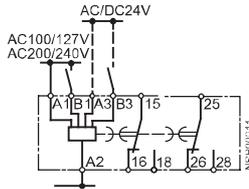
ON-delay and OFF-delay
