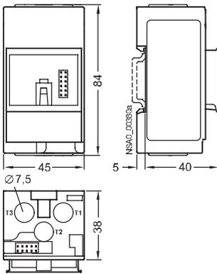
3UF7 102 current measuring module (straight-through transformer)
