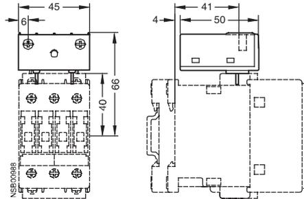
**3RT19 16-2D solid-state time-delay blocks, OFF-delay**
