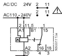
Flashing, starting with interval (D)
