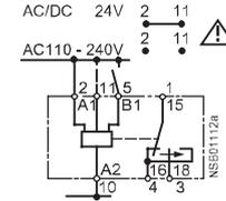
Pulse-forming with auxiliary voltage (B)
