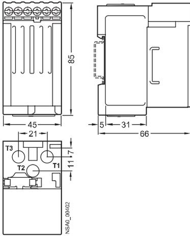
**3UF7 112 current/voltage measuring module (straight-through transformer)**
