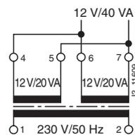
The 12 V outputs must be switched in parallel or in series. Our example shows the 4AC3 140. In parallel connection, they can be used for 12 V/40 VA, in series connection for 24 V/40 VA. In these types of circuits, the PTC resistor ensures full protection of the transformer.
