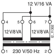
The 12 V outputs must be switched in parallel or in series. Our example shows the 4AC3 616. In parallel connection, they can be used for 12 V/16 VA, in series connection for 24 V/16 VA. In these types of circuits, the PTC resistor ensures full protection of the transformer.
