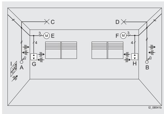
Modification of the installation for shared operation of lighting and shutters/blinds from various operating points.
