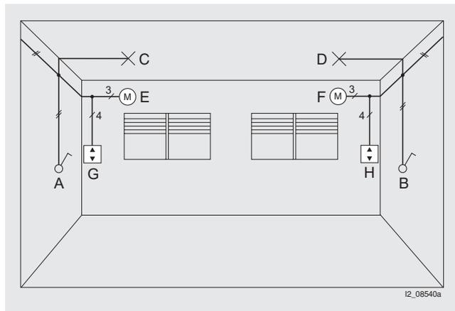
Example of a conventional installation with lighting and electrically operated shutters/blinds.
