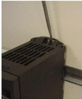
1. To disengage the release mechanism of the inverter, insert a screwdriver into the release mechanism.
