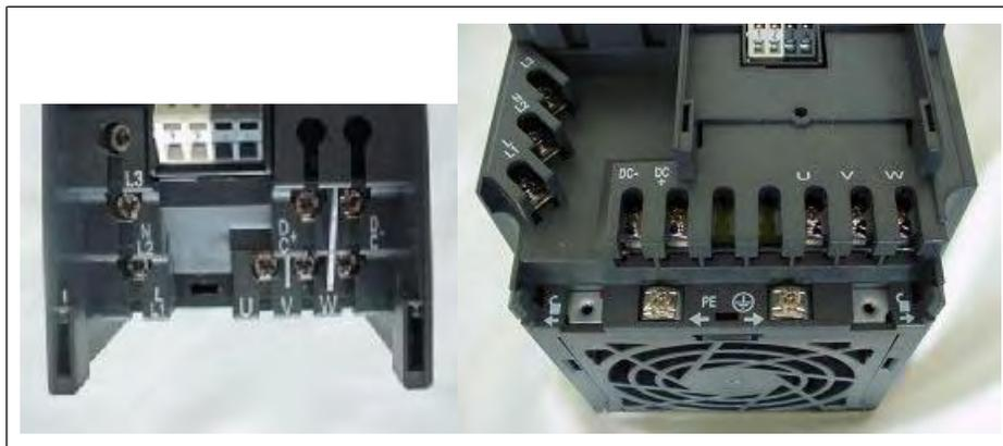
Figure 2-5 MICROMASTER 420 connection terminals
