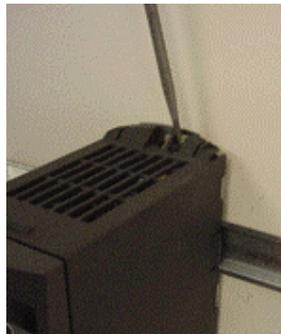
1. To disengage the release mechanism of the inverter, insert a screwdriver into the release mechanism.
