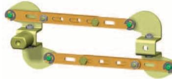
Provides for simultaneous switching of two circuit breakers/switch disconnectors. Parallel switching can be used between two 3VT2 circuit breakers or between 3VT2 and 3VT3 circuit breakers. Each circuit breaker must be equipped with a rotary operating mechanism and at least one with a knob.
