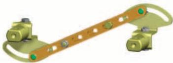
Provides mechanical interlocking of two circuit breakers/switch-disconnectors so that they cannot both be tripped simultaneously, but only one of them at a time. Both circuit breakers may be turned off simultaneously. Interlocking can be used between two 3VT3 circuit breakers or between 3VT3 and 3VT2 circuit breakers. Both circuit breakers must be furnished with a hand drive (at least one with a manual operating mechanism and knob), see page 4/48.
