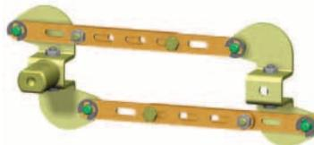
Provides for simultaneous switching of two circuit breakers/switch-disconnectors. Parallel switching can be used between two 3VT3<sup>1)</sup> circuit breakers or between 3VT3 and 3VT2 circuit breakers. Each circuit breaker must be equipped with a manual operating mechanism and at least one with a knob, see page 4/48.
