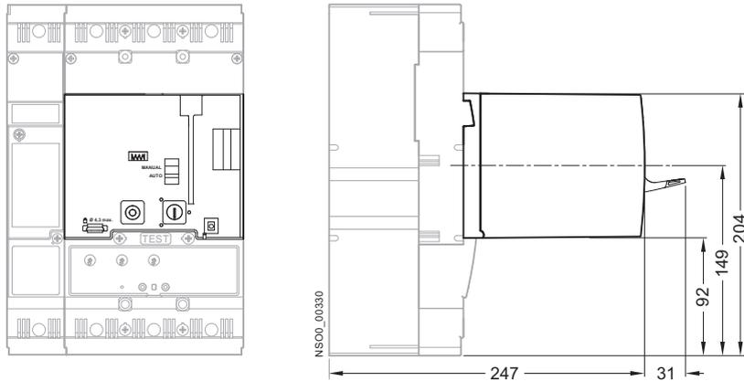
Opening dimensions in cabinet door for external operations counter
