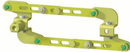
Mechanical interlocks for parallel switching are for simultaneous switching of two circuit breakers. Parallel switching can be used between two 3VT1 circuit breakers. Each circuit breaker must be furnished with a manual operating unit and at least one with a knob (see page 2/25). In order to use parallel switching, it is absolutely necessary to comply with the dimensions shown in the figure and given in the table.
