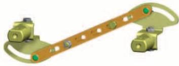
Provides mechanical interlocking of two circuit breakers/switch disconnectors so that they cannot both be tripped simultaneously, but only one of them at the same time. Both circuit breakers may be turned off simultaneously. Interlocking can be used between two 3VT2 circuit breakers or between one 3VT2 and one 3VT3 circuit breaker. Both circuit breakers must be furnished with a rotary operating mechanism (at least one with a rotary operating mechanism and knob).
